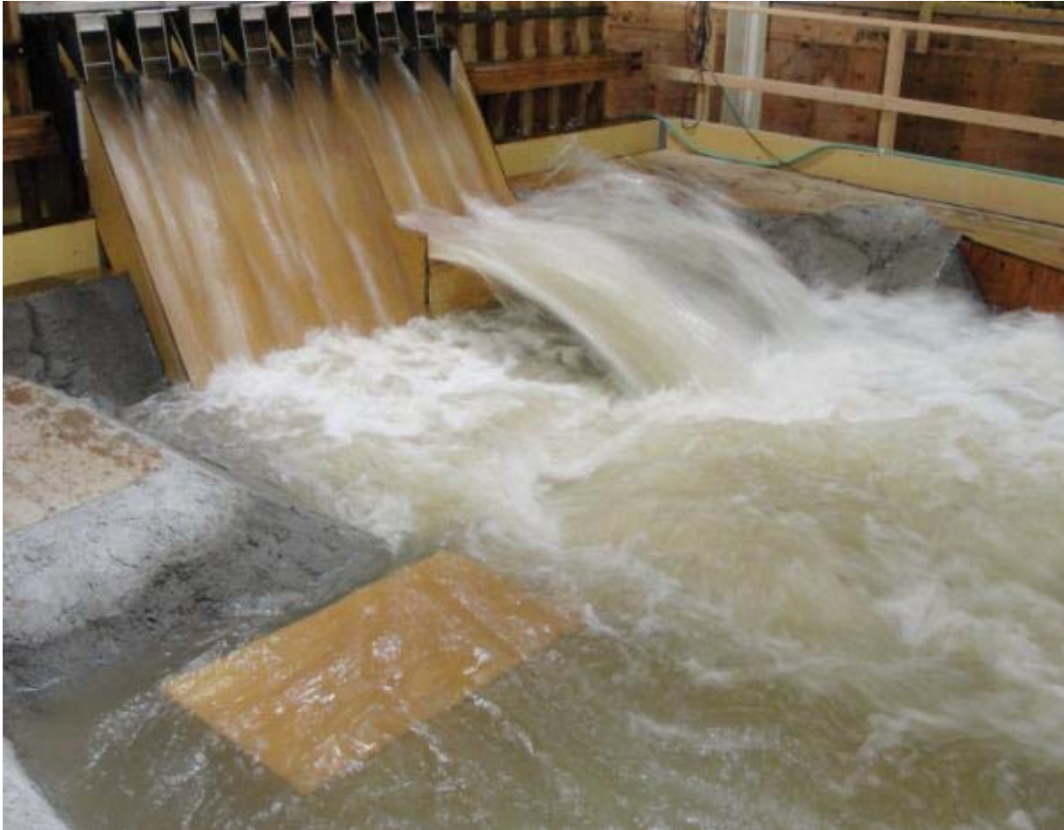
Figure 3-3: Emergency Spillway Flip Bucket Trajectory, 1:48 model
